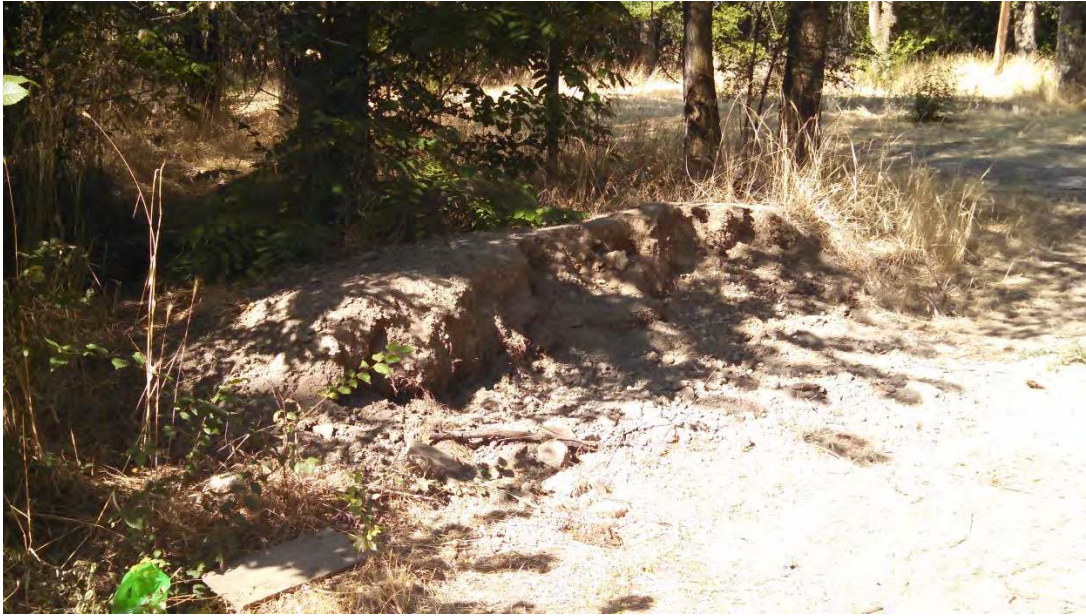
Photograph 26: Fill dirt pile observed near eastern site corner. Pile was comprised of silty sand. Staining was not observed and odors were not noted in the soil pile. View looking to the south.
